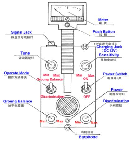
searching, press and release the push button immediately to reset the threshold.
